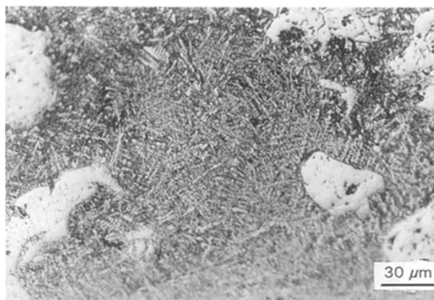
Figure 1 Photomicrograph of a cross-section of the LSA zone of Armco iron.
